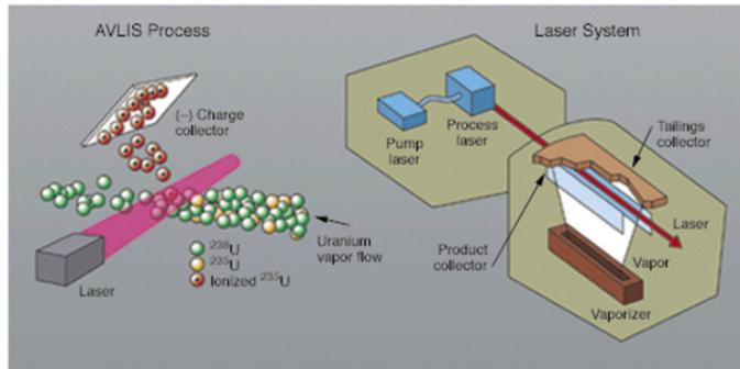
In the laser system used for the LIS uranium enrichment process (right), electrons from the  $^{235}\text{U}$  atoms are separated (left), leaving positively charged  $^{235}\text{U}$  ions that can be easily collected for use. Figure 1: Simplified diagram of the AVLIS system [2]
