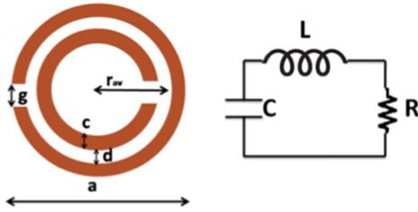
Figure 1. Schematic of a double-turn split-ring resonator and equivalent RLC tank circuit of a single split-ring resonator.<sup>2</sup>
