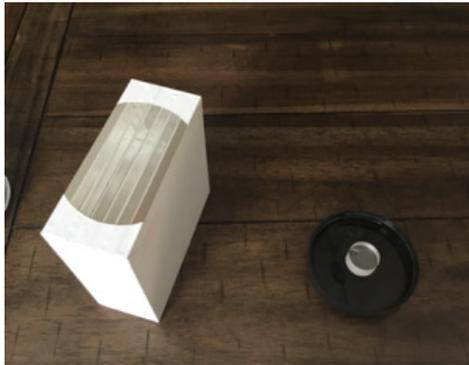
Figure 3. Composite ZEBRA (left) vs. Non-composite (single crystal) Lu<sub>2-x</sub>GdxSiO<sub>5</sub> (LGSO). [3]
