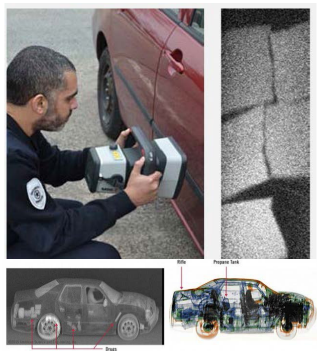
Figure 8. Top Left: Rapiscan Mini Z. Top Right: Hidden contraband currency. Bottom Left: Transmission Scan of Vehicle with rifle and propane tank. Bottom Right: hidden drugs. Images courtesy of Laurus Systems.
