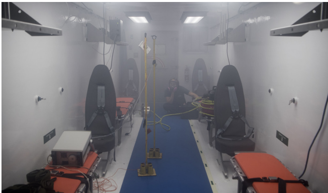
Figure 4: Portable Bio-Containment Module (PBCM) is shown being tested for Aerosol Integrity on a C-17 [18]
