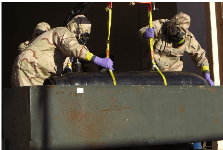
Figure 2. Workers wearing CW protective suits remove a chemical weapon from a transportation container during the process of destroying the munition.
