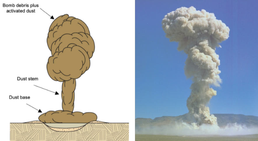
Figure 8: Characteristic debris cloud in a Regime 6 event (left) and the cloud from the Johnny Boy test, a shallow-buried device with \text{SDOB} of -2.4 \text{ ft/kt}^{1/3} .
