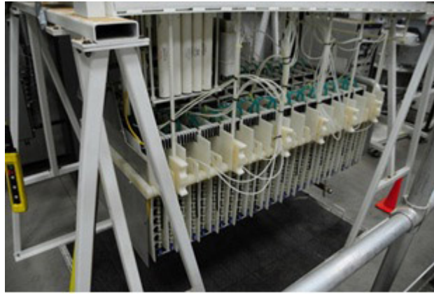
Figure 5b. The Marx generator named after its inventor Erwin Otto Marx is used to drive the required Reltron tube.
