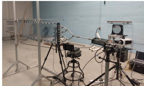
FIGURE 4: Shock tube, displaying to the right the shock wave generation apparatus that propagates into the rectangular tube, left. Although currently clean for an ideal test, material piled on the floor allows for non-ideal tests.
